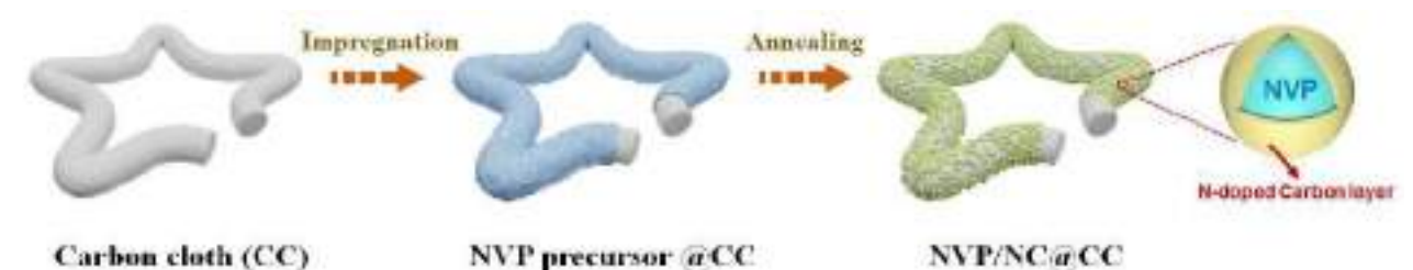
Figure 1. Schematic illustration for the formation of the NVP/NC@CC flexible electrode.
