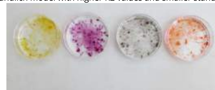
Figure 1. Sol-gel color change after heavy metal interaction.
