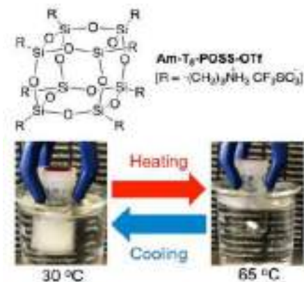
Figure 1. Temperature-responsive behavior of Am-T8-POSS-OTf.
