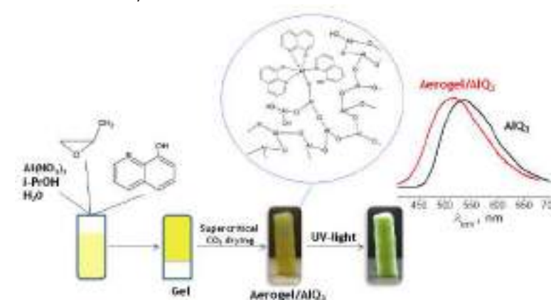
Figure 1. The general synthetic scheme for Al 2 O 3 aerogels, modified by AlQ 3 .
