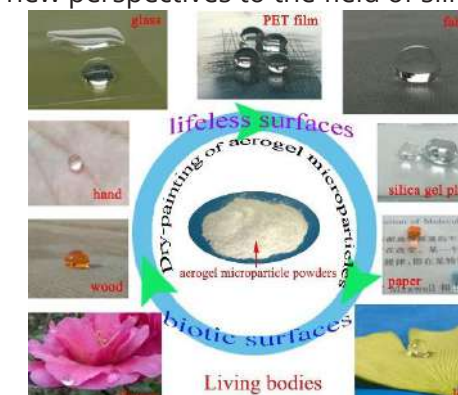
Figure 1. The application of silica aerogels in superhydrophobization of living bodies.
