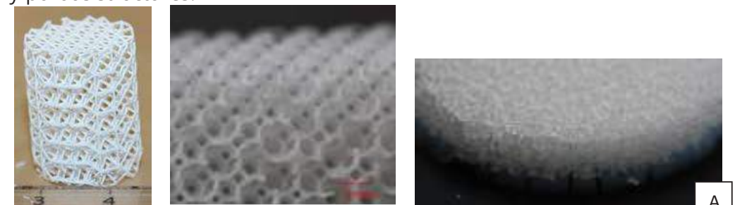
Figure 1. 3D-printed ceramic sample with 200-micron features prepared using stereolithography printer. Sample A is a 3D-structured silica aerogel.
