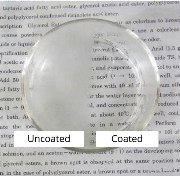
Figure 2. Anti-fogging property of sol-gel coating from silane coupling agent containing EO-extended polyglycerin.
