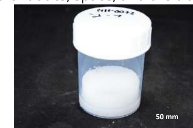
Figure 1: Wet gel body of homogeneous alumina silica (molar ratio 1:1).
