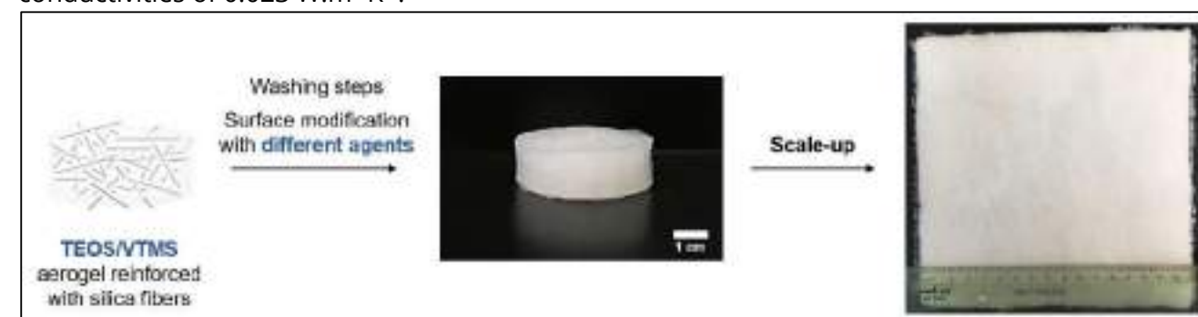
Figure 1. Scheme of the scale-up of TEOS/VTMS aerogels reinforced with fibers, and modified with HMDZ prior to APD.
