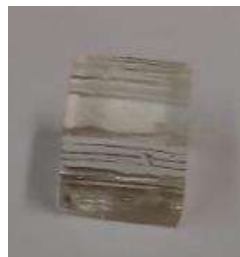
Figure 1. Photo of sol-gel element printed by Ink-jet 3D printer.
