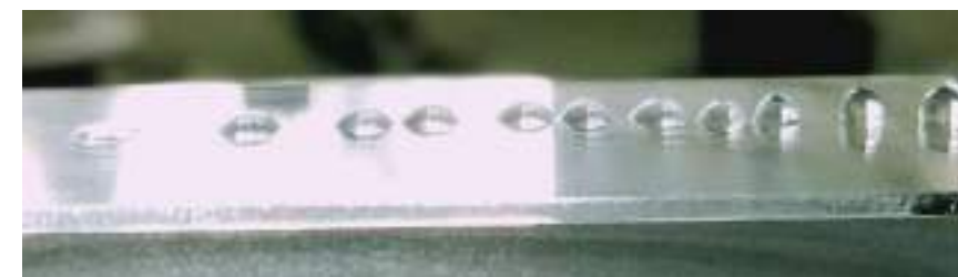
Figure 1. Example of a Sol-Gel coating showing a wettability gradient.
